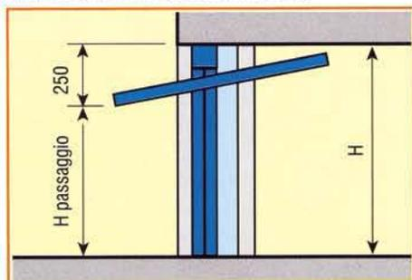
**SCHEMA DI MONTAGGIO PORTA OLTRE LUCE** *Installation diagram of door outside reveal*
