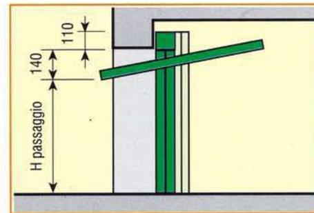
**SCHEMA DI MONTAGGIO PORTA IN LUCE** *Installation diagram of door within reveal*
